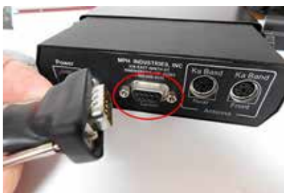
The GPS Speed Interface connects via a supplied connector which plugs into the in-car video/RS-232 port.
