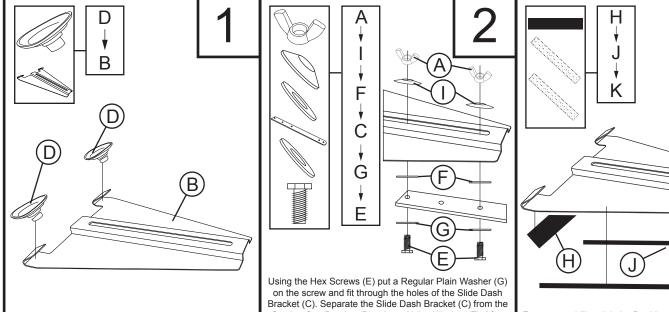
Bracket (C). Separate the Slide Dash Bracket (C) from the Suction Cup Bracket (B) using a Nylon Washer (F). After joining the two brackets together, add a Spring Disc (I) and secure with a Wing Nut (A) on each screw.
