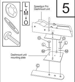
Remove 2 wingnuts and washers as shown. Use screws (O) and washers (L,M) to attach dashmount unit mounting plate to (C). Re-attach Speedgun Pro dashmount unit to attached mounting plate using provided wingnuts and washers.
