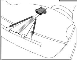
Put the finished bracket into the car on the dash. Be sure to secure the Suction Cups (D) to the window and then stabilize with the Dual Lock Strips (J,K), if you choose to use them. Mount the Speedgun Pro to the bracket and adjust the Slide Dash Bracket to fit.
