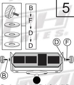
Place the radar unit onto the Display Bracket (A). Fit a Regular Washer (F) onto a Stud Knob (B). Place a Nylon Washer (D) against the REgular Washer (F) and another between the radar unit and the Display Bracket (A). Repeat for other side.
