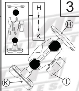
Using the Joint Swivel (I) fit both Ball Joints (H)(K) onto either side. Tighten the Joint Swivel (I) to safely hold parts together, do not tighten.
