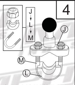
Once the bracket is firmly built, fit Bushing (L) in the middle of the U-Bolt (M). Take the U-Bolt (M) and fit it under the handle bar of the motorcycle so the Bushing (L) is directly on the surface. Place the bracket on top of the U-Bolt (M) through the holes on the Bottom Ball Joint (K). Secure using the Nut (J) provided. Tighten in place.
