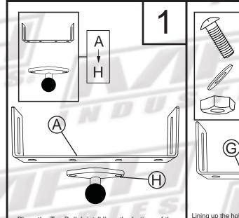
Place the Top Ball Joint (H) on the bottom of the Display Bracket (A), lining up the two bolt holes.
