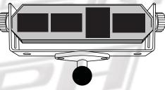
When Finished, the radar unit can be adjusted by loosening the Stud Knobs (B) and moving the radar unit in the direction preferred by the person.
