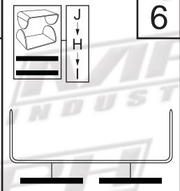
Pick a place in the vehicle to mount the bracket. Take the Dual Lock Pad (H)(I) and remove the adhesive covering to put onto the bottom of the Antenna Windshield Bracket (J). Mount in the area of the vehicle by removing the bottom adhesive strip.
