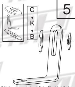
With the antenna in hand, fit the Shoulder Washer (C) onto the stud of the antenna. Put through the slot of the Angle Slotted Bracket (K) and fit a Nylon Washer (B) onto the stud separating the bracket from the knob included with the antenna kit.
