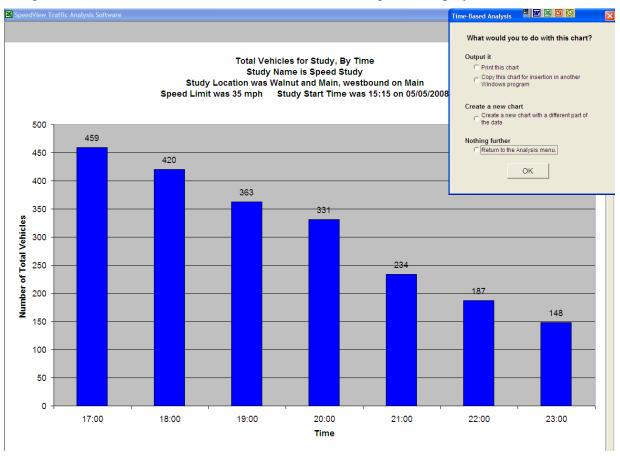
Each bar shows the total number of vehicles that the radar counted during the previous hour. For example, the 17:00 bar shows that 459 cars passed the radar in the westbound direction on Main Street between 16:00 and 17:00 on 5/5/08.
