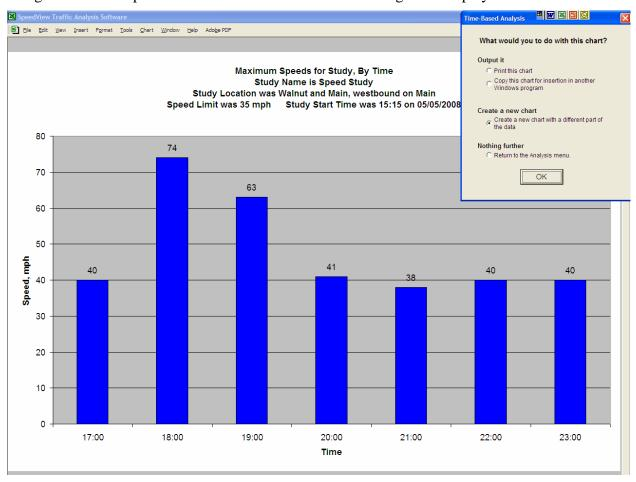
Each bar shows the fastest vehicle speed that the radar saw during the previous hour. For example, the 17:00 bar shows that the fastest vehicle that passed the radar in the westbound direction on Main Street between 16:00 and 17:00 on 5/5/08 was traveling 40 mph.
