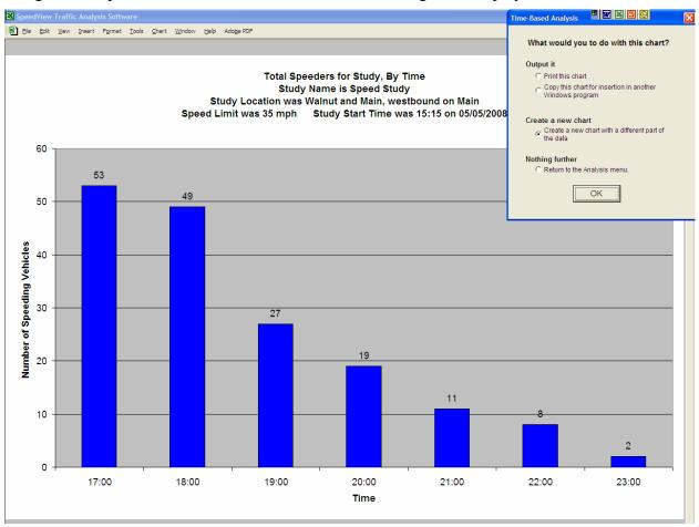
Each bar shows the total number of speeders that the radar counted during the previous hour. For example, the 17:00 bar shows that 53 cars exceeding the 35 mph speed limit passed the radar in the westbound direction on Main Street between 16:00 and 17:00 on 5/5/08.
