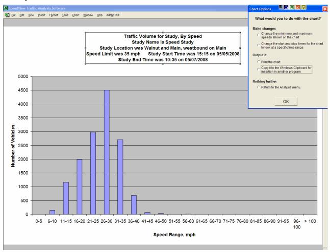
The graph shows you the traffic volume for the entire study, based on the vehicle speeds.
