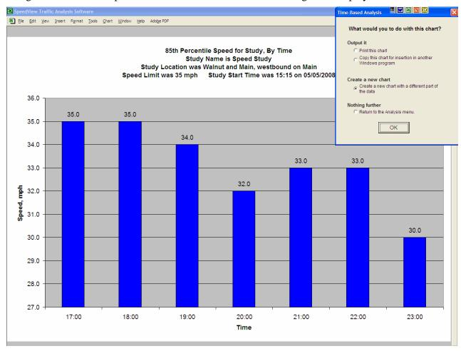
Each bar shows the statistical 85<sup>th</sup> percentile speed of the traffic during the previous hour. For example, the 17:00 bar shows that the 85<sup>th</sup> percentile speed of the westbound traffic on Main Street between 16:00 and 17:00 on 5/5/08 was traveling 35 mph.
