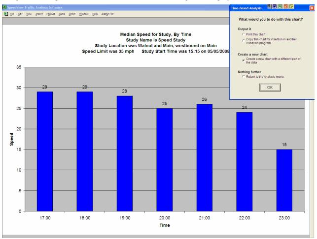
Each bar shows the statistical median speed of the traffic during the previous hour. For example, the 17:00 bar shows that the median speed of the westbound traffic on Main Street between 16:00 and 17:00 on 5/5/08 was traveling 29 mph.
