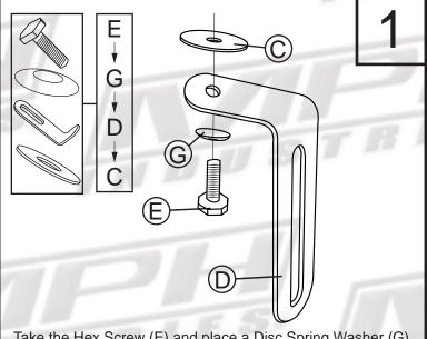
Take the Hex Screw (E) and place a Disc Spring Washer (G) on to the stud. Fit through the hole of the Angle Bracket (D) followed by a Nylon Washer (C).
