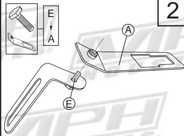
Thread the Visor Bracket (A) to the Hex Screw (E). Tighten to secure the brackets together.
