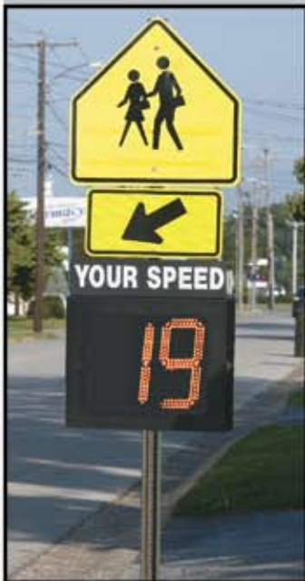
Speed Guardian with top-mounted "Your Speed" sign, mounted on perforated post
